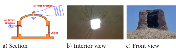
Figure 6. A windward ventilator called Kolak in Sistan local language (source: Sargazi et al., 2022)
