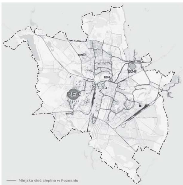
Fig 4. Heat distribution network diagram superimposed on city map
