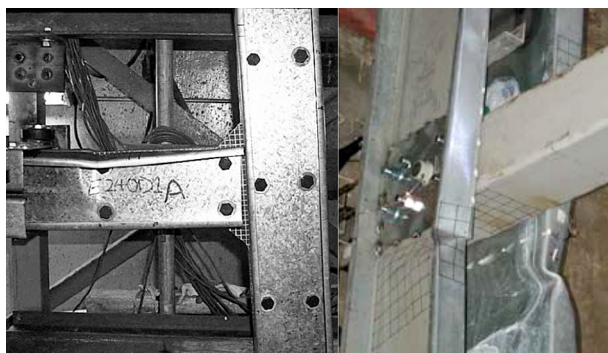
Fig. 7. Local buckling in beam and column sections (Uang et al. 2010; Wong, Chung 2002)
