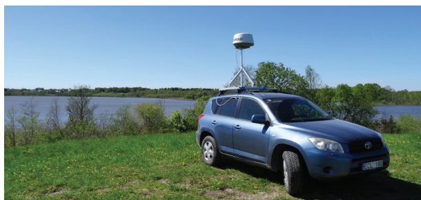
Figure 3. SIMRAD 4G TM radar mounted on SUV
