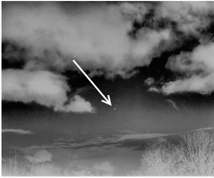
Figure 1. UAV at 200 m. detected by LWIR (long wave infra-red, 20 mm focal distance) camera at clear sky behind DJI Phantom 3
