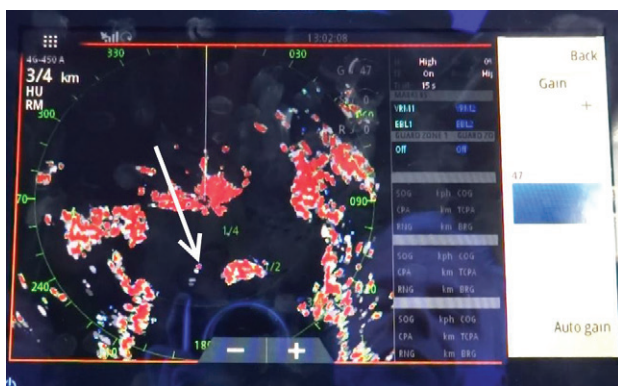
Figure 9. DJI Phantom detection over the lake using SIMRAD 4G™ radar
